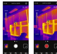
Slide the camera icon left/right to enter the video mode. Tap video icon to record videos, and the recording duration will be displayed in the lower right corner. Tap the video icon again to end the recording.
