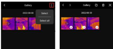
Tap an image/video to enter an interface where users can preview/share/delete/edit (image only) this image/video, view its PIP/fusion mode or detailed information (filename, date, time, resolution, Hi spot, Lo spot, center spot, mode, emissivity).
